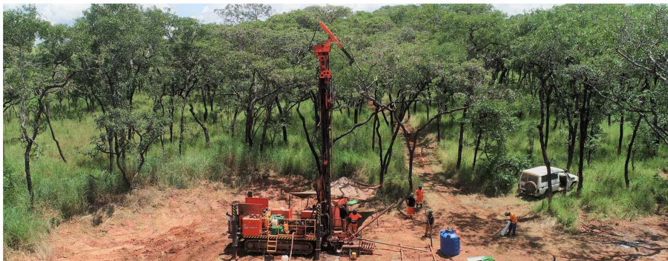
Delineation drilling at kimberlite L071
