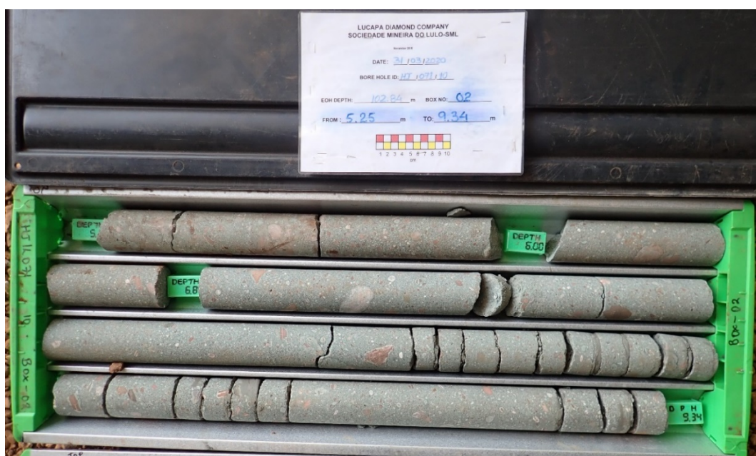
Figure 1: Fresh high interest volcanoclastic kimberlite material (at 5m depth) in drill core from L071
