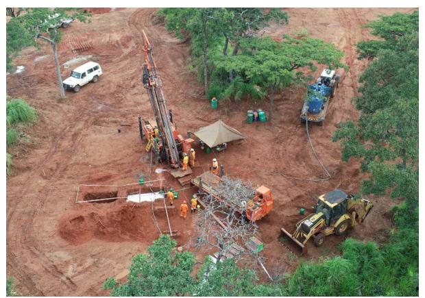
Figure 1: Drilling of kimberlite L030 with the mobile Hanjin rig in the Canguige catchment area at Lulo
