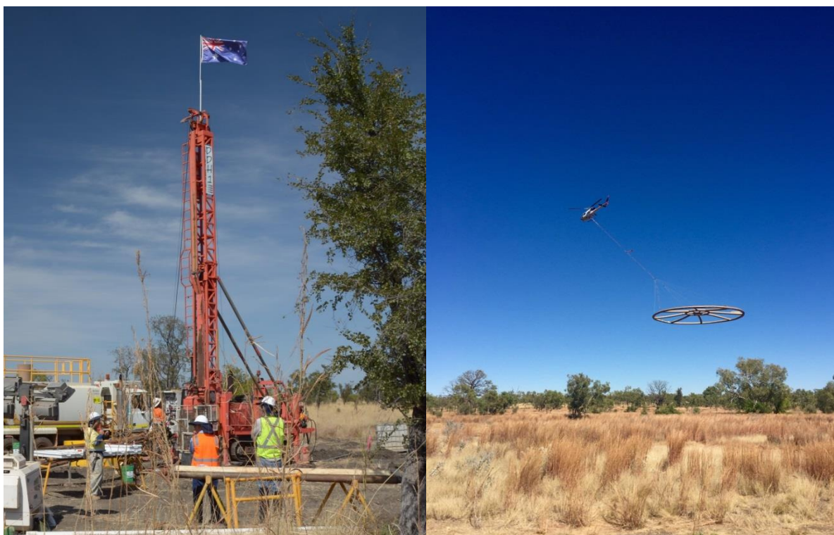
Drilling at the Little Spring Creek discovery and flying of the TDEM survey across the entire Brooking project
