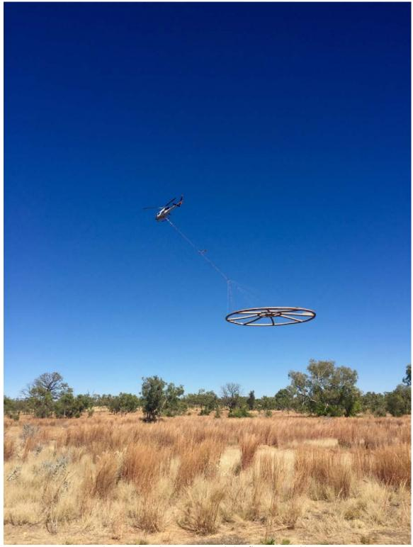
Figure 3: The Xcite TDEM survey being flown at Brooking
