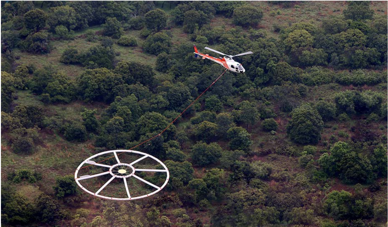
Figure 5: Picture of the Xcite TDEM technology scheduled to be flown over the entire 118km 2 Brooking project later in June 2018
