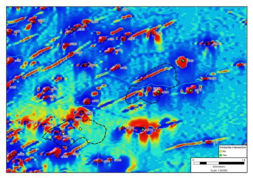
Figure 2: Magnetic target identified at L164 from aeromagnetic survey
