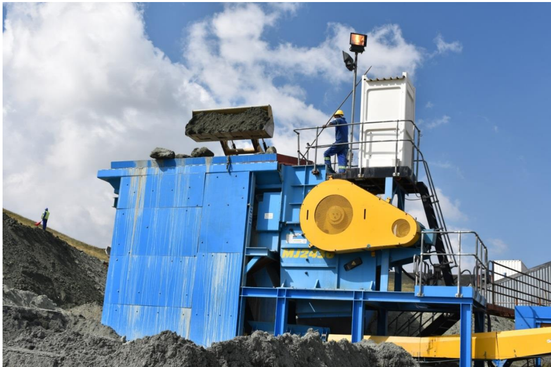
Feeding the primary crusher of the re-commissioned bulk sampling plant and infrastructure at Mothae
