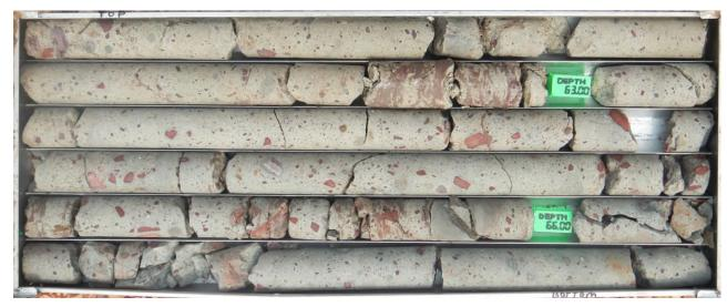
Figure 3: Kimberlite core intersected in E4
