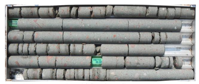
Figure 2: Kimberlite core intersected in G510
