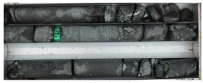
Figure 4: Kimberlite core intersected in E6
