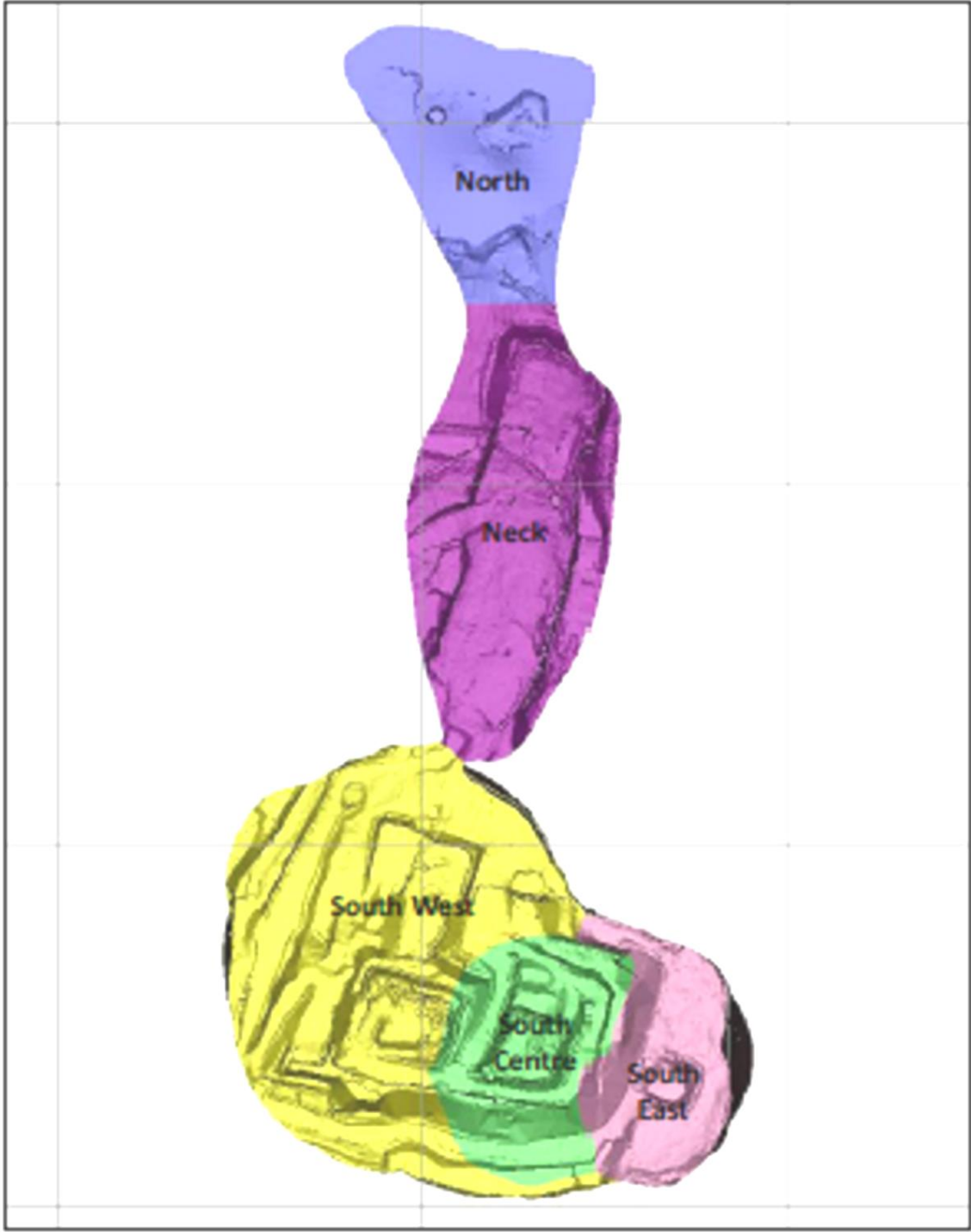
Figure 14-11 Plan view of the Mothae three-dimensional geological model at surface showing the five major internal geological kimberlite domains
