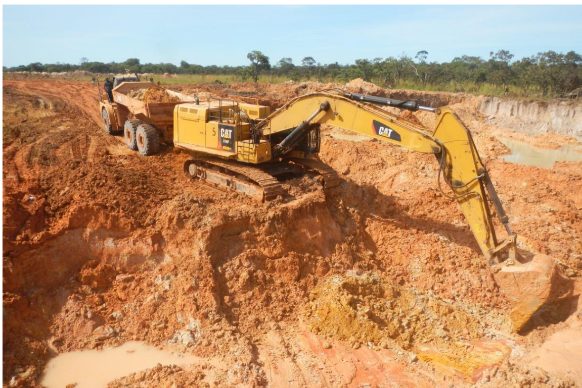
Excavation of alluvial gravels from Lulo Mining Block 8
