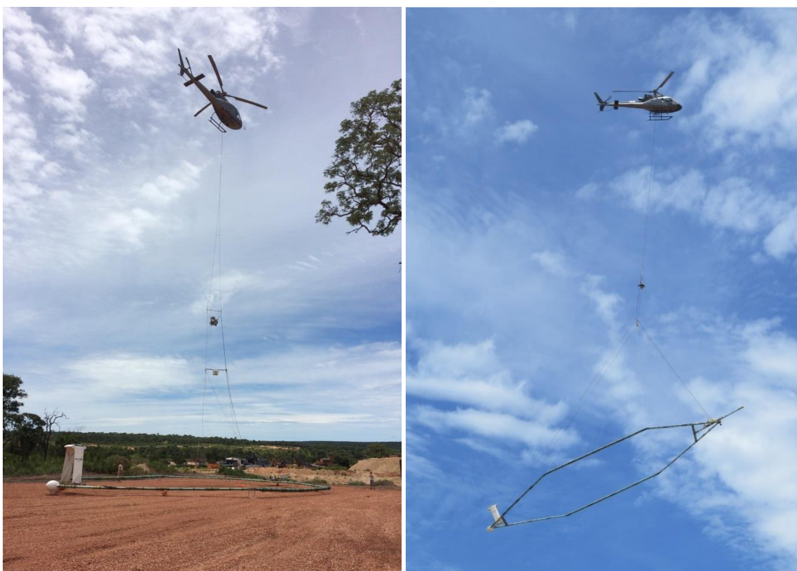
The helicopter-borne TDEM survey flown over the Cacuilu River valley block at Lulo
