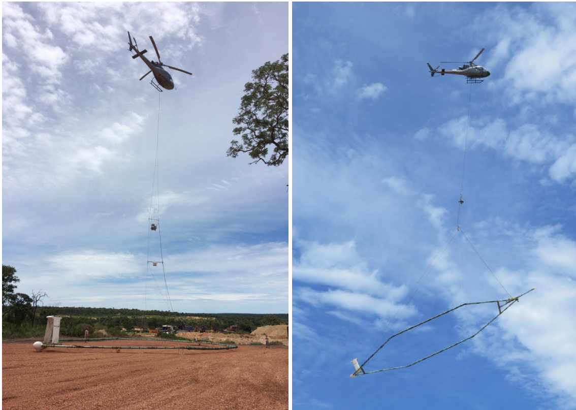
The helicopter-borne TDEM survey over the Caculo River valley block at Lulo
