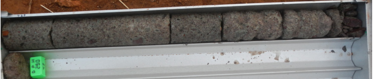
Figure 4: Drill core from L13 (Hole: RS/013/04, Depth: ~27.90m - 29.00m)
