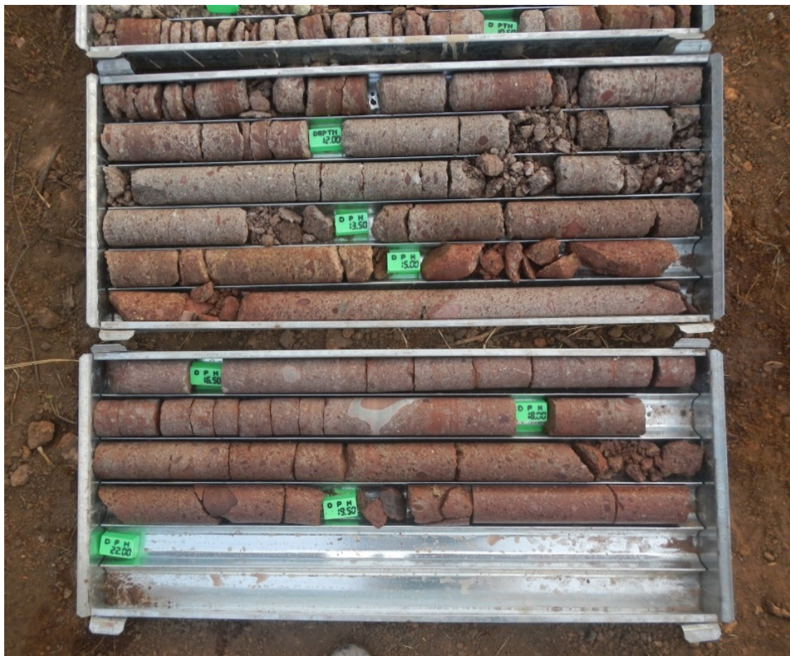
Figure 1: Core from the first hole drilled at the L14 kimberlite discovery, within ~2km and upstream of Mining Block 8 on the Caculo River (Hole: HJ/014/01, Depth: ~10.00m – 22.00m)
