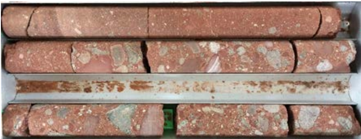
Figure 2: Core tray 11 from L15 (RS/015/01), illustrating the fining-upward sequence from coarse- to fine-grained RVK in the 35.5m and 38.5m interval
