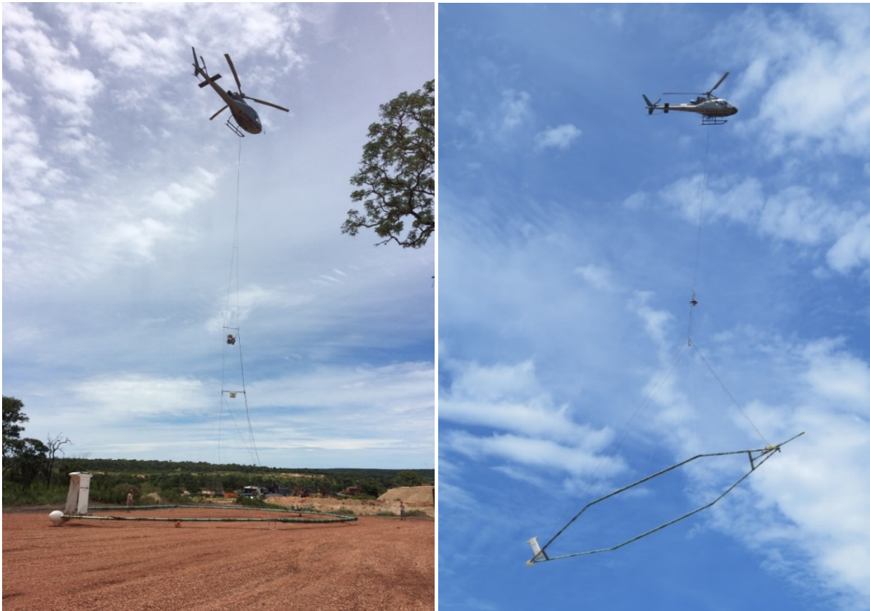
The helicopter-borne TDEM survey over the Caculo River valley block at Lulo is now complete
