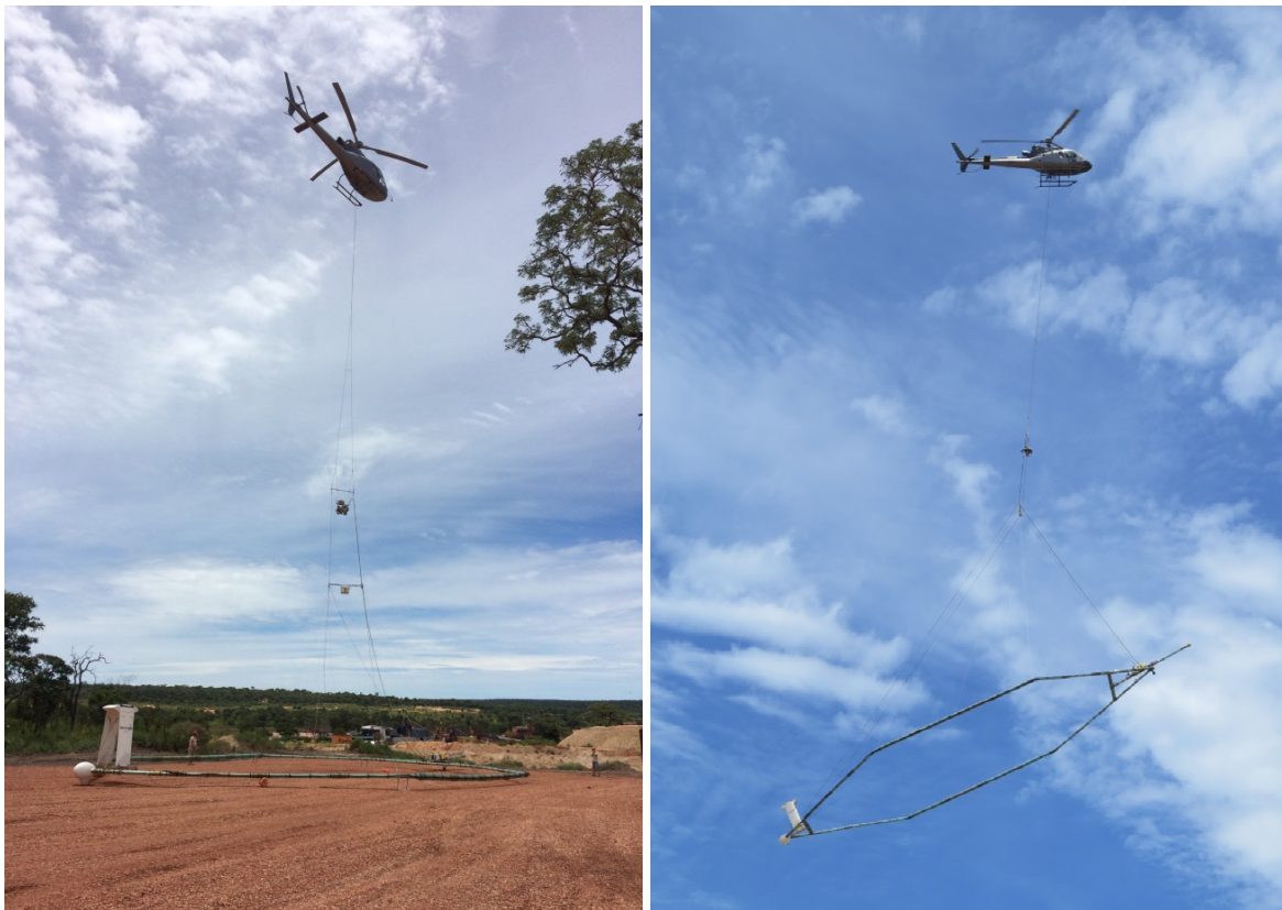
The helicopter-borne TDEM survey over the Caculo River valley block at Lulo is about 80% complete
