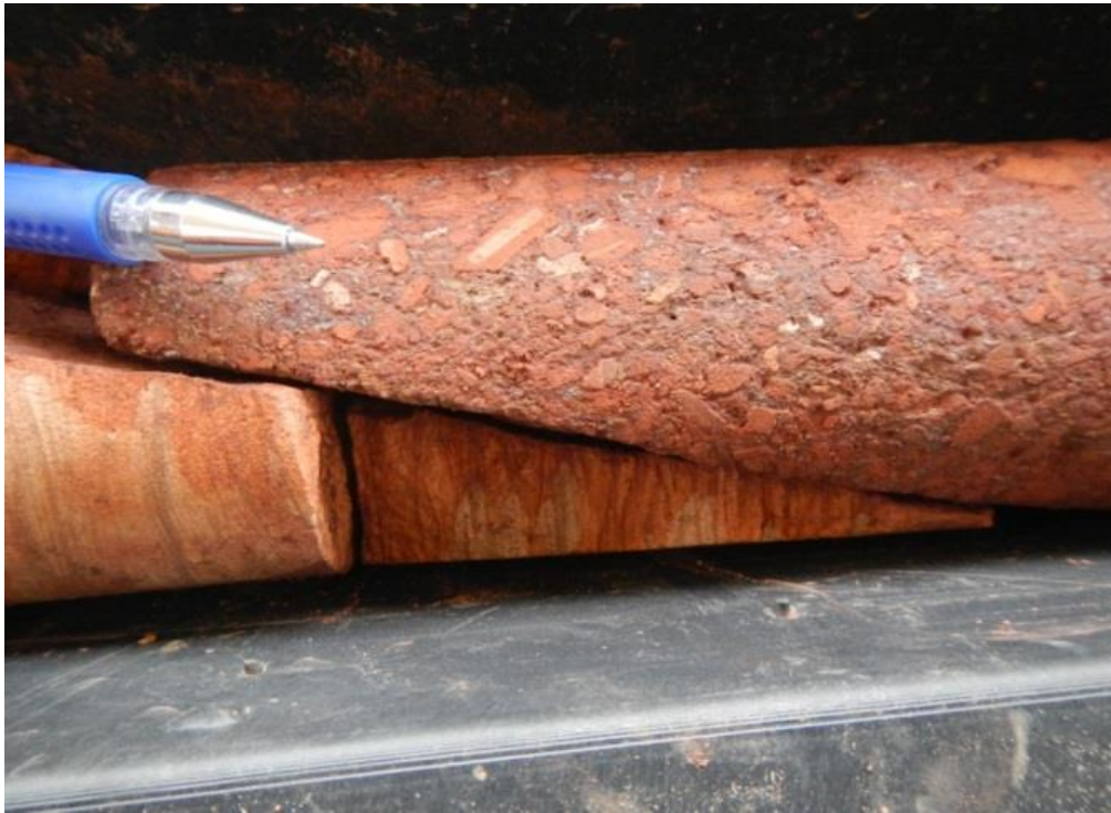
Coarse kimberlite in drill core from L171 with clear contact at 39.7m
