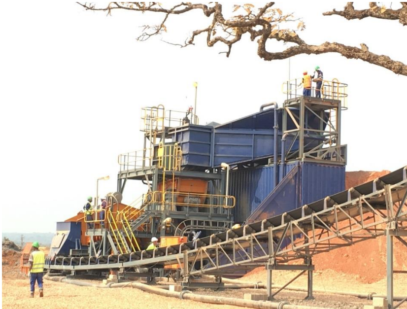
New wet front end installed at the 150 tonne per hour Lulo plant during the Quarter
