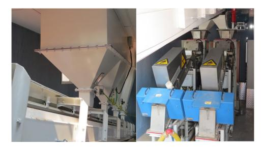
Figure 5: New double pass Flowsort x-ray diamond recovery machines installed to improve capacity and efficiency of diamond recoveries
