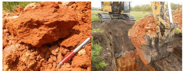
Figure 9: Excavator pitting over the kimberlite target area (left) and in-situ RVK material (right) recovered from pits adjacent to the expanded Mining Block 8
