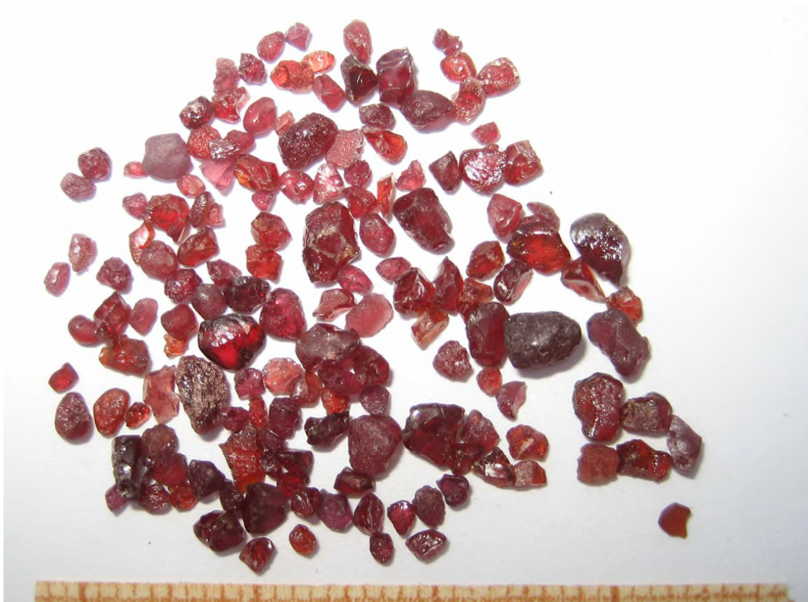
Figure 1: Coarse garnets (kimberlite indicator minerals) recovered from Mining Area 8 at Lulo, within ~300 metres of the E259 kimberlite target
