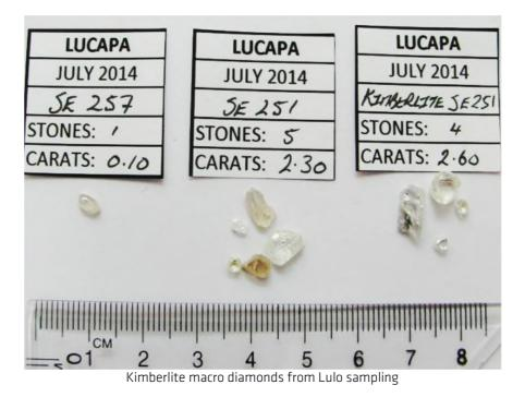
A total of 12 diamonds have been recovered from the L251 pipe (Figure 2 and Table 1). Of those 12 diamonds, five have been confirmed as Type IIa stones after testing with a Yehuda ZVI colorimeter.
