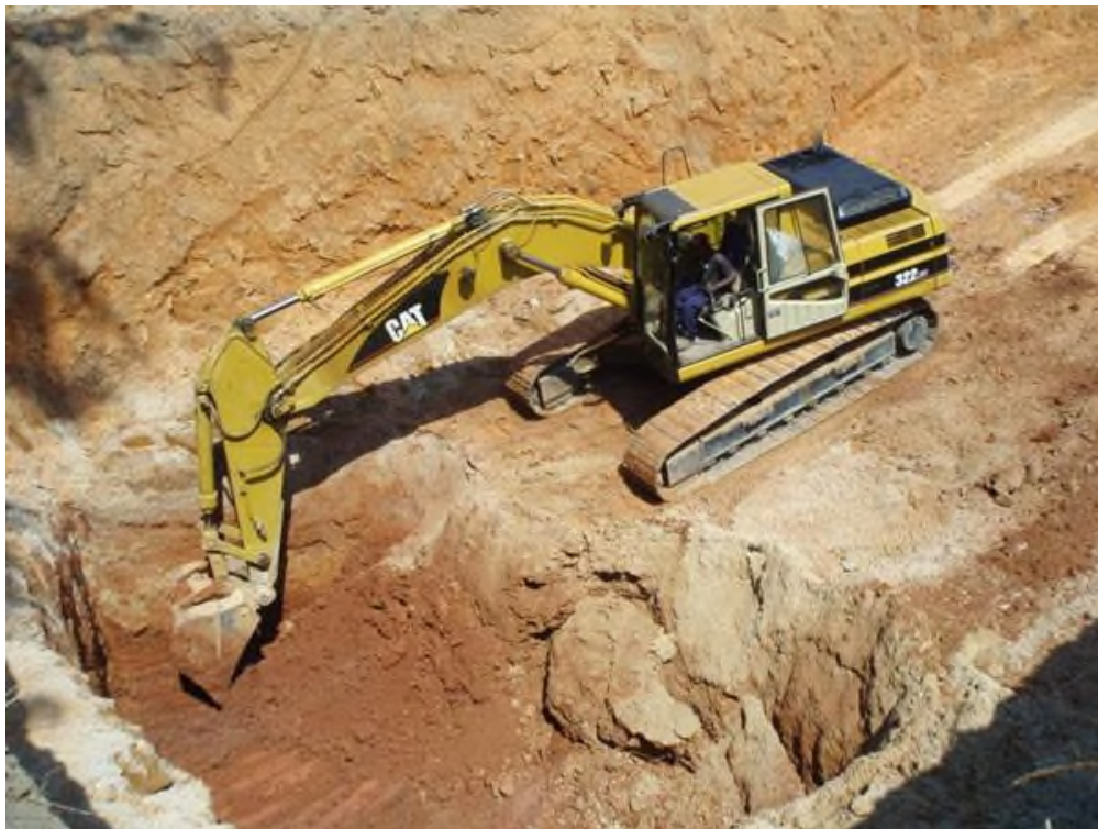
Excavating kimberlite samples from the diamond-bearing Se251 kimberlite pipe
