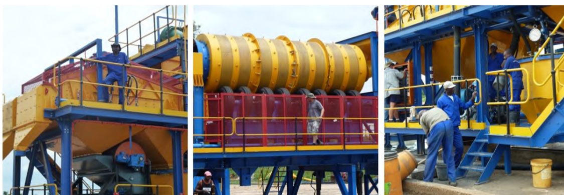
Lucapa's Dense Media Separation diamond plant
