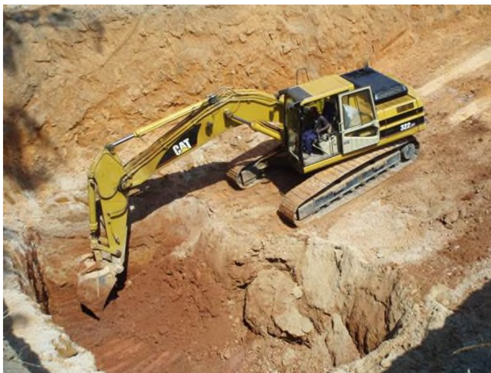
Excavating sample from diamondiferous kimberlite pipe Se251 at Lulo
