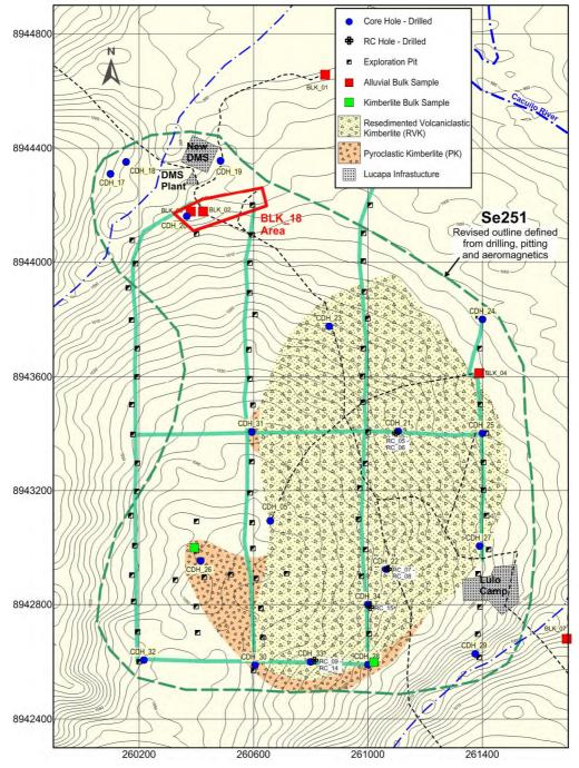
Figure 1: Se251 kimberlite and location of BLK\_18 and new DMS plant
