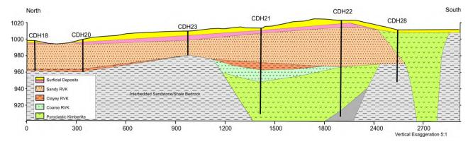
Figure 2: North-south drill section through kimberlite Se251
