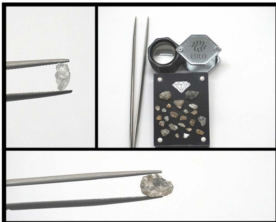
Picture: Bulk sample from KBS/164/02 showing the 23 diamonds recovered and the largest stone (bottom) recovered from the sample, a 2.38 carat diamond as well as a 0.71 carat diamond (top left)
