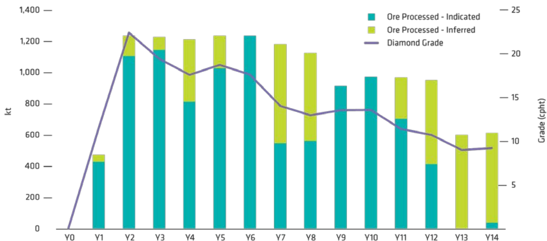
Graph: Annual production target, diamond grade and Indicated and Inferred Resource contribution
