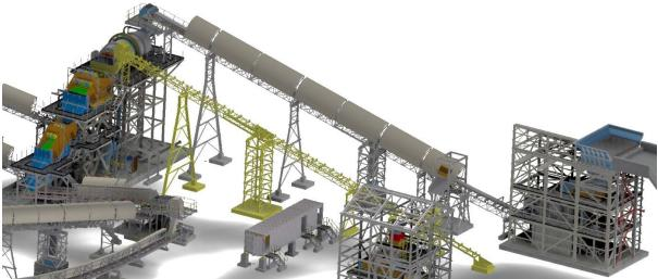
Bypass conveyor modification (yellow) to plant to reach 1.6Mtpa processing capacity Primary crusher (far right) is also being upgraded
