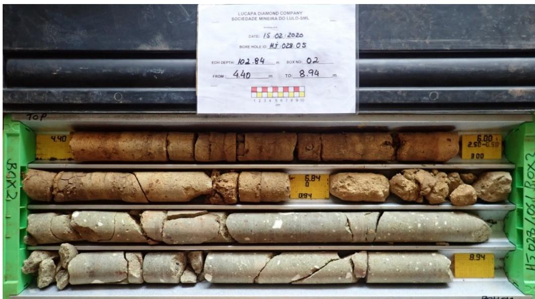
Figure 3: Core from drilling of first of the top-rated pipes in the Canguige catchment (L028) showing shallow intersection of kimberlite material
