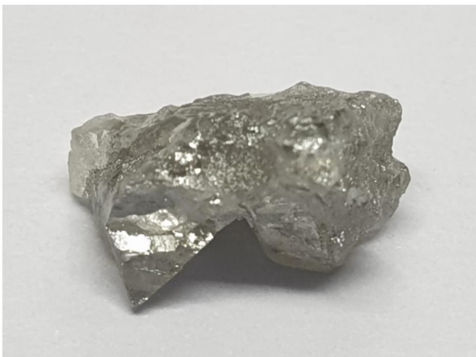
Figure 2: 2.05 carat diamond recovered from kimberlite L104 bulk sample
