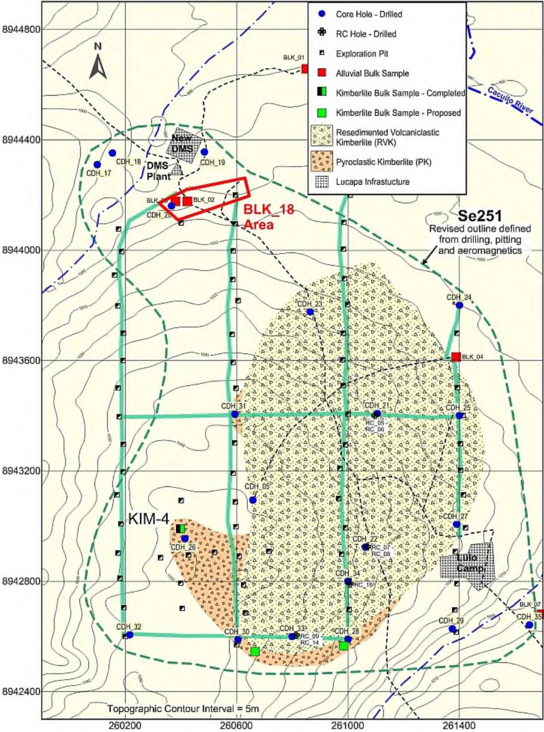
Figure 1 – Se251 Kimberlite – Geology and Sampling
