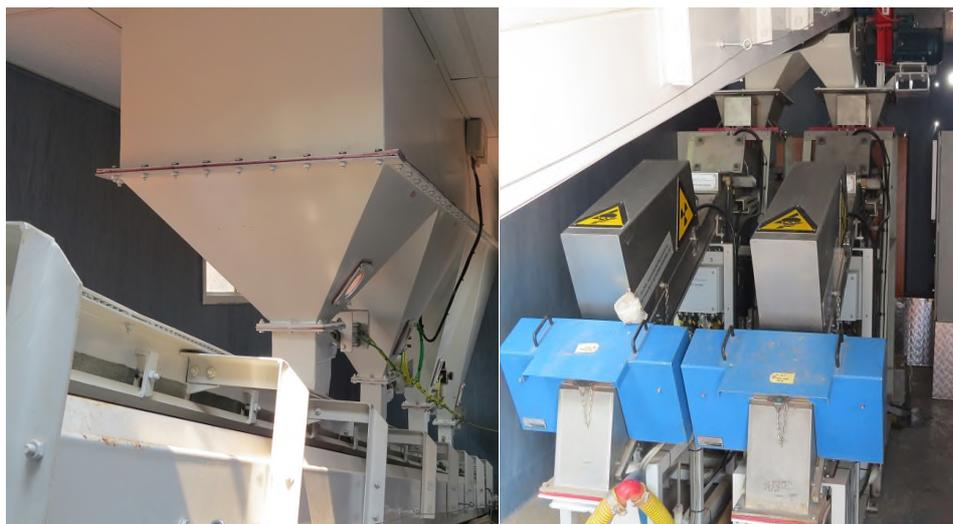
Figure 5: New double pass Flow-sort x-ray diamond recovery machines installed to improve capacity and efficiency of diamond recoveries
